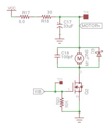
A vibration motor (M1) is a common component implemented in consumer electronics to provide haptic feedback. The above analog circuit represents one type of motor implementation. For the following questions, you may assume VCC = 2.9V. VIB is sourced from the tri-state output of a microcontroller. VIB is switched to 2.9V for one second, then switched to GND for 20 seconds, and repeated indefinitely.
